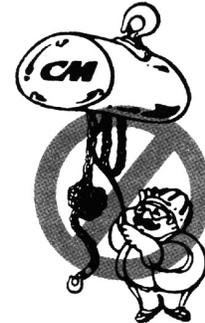
**! WARNING** — DO NOT PULL AT AN ANGLE. BE SURE HOIST AND LOAD ARE IN A STRAIGHT LINE.
