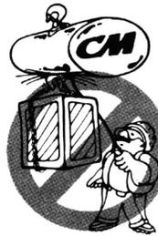
Do not use load chain as a sling. Such usage damages the chain and makes the limit switch setting ineffective.
